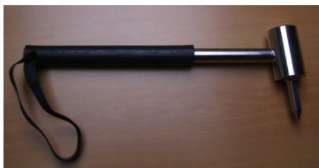
Pre-drilling hammer (weight : 2.5kg / Length : 50cm)
