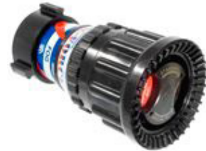
MAXFORCE tip 4000- 2000 l/min, 4 and 7 bar, 3 kg Ref. I12.42.012
